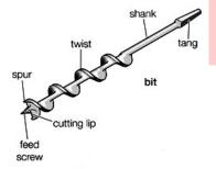
Auger, tool (or bit) used with a carpenter's brace for drilling holes in wood. It looks like a corkscrew and has six parts: screw, spurs, cutting edges, twist, shank, and tang.
